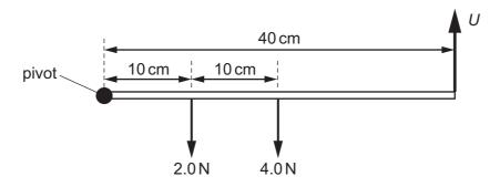
An upward force *U* is needed to keep the beam horizontal.
