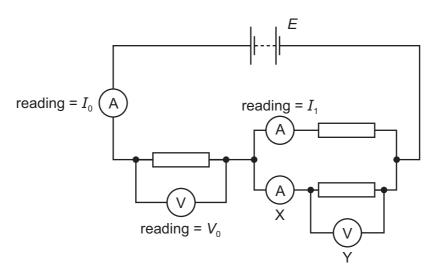
The readings of two ammeters and a voltmeter are shown.
