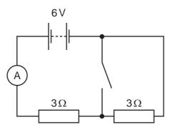
What is the reading on the ammeter when the switch is open, and the reading when it is closed?
