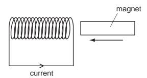
The magnet is then pulled out quickly from the same end of the coil.
