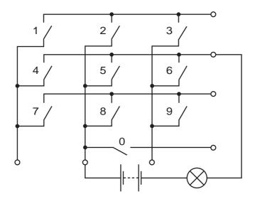
Which single switch can be pressed to make the lamp light?
