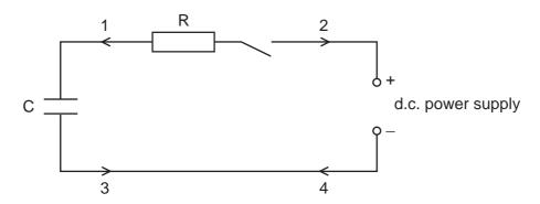
Which arrows show the direction of the conventional current when the capacitor is charging?
