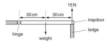
When the trapdoor is closed, the ledge exerts an upward force of  $15\,\mathrm{N}$  on the trapdoor. The gravitational field strength is  $10\,\mathrm{N/kg}$ .
