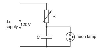
The neon lamp lights when the p.d. across the capacitor C reaches 110 V. C then discharges through the neon lamp. When C has discharged, the lamp goes out and the p.d. across C slowly increases once more.
