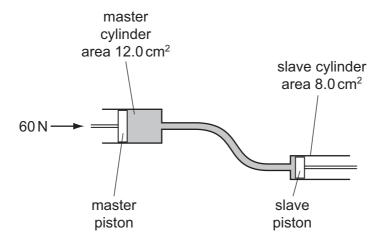
The cross-sectional area of the master cylinder is  $12.0~\text{cm}^2$  and the cross-sectional area of the slave cylinder is  $8.0~\text{cm}^2$ . The force applied to the master piston is 60~N, producing a pressure of  $5.0~\text{N/cm}^2$ .
