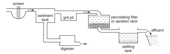
The sewage works will not perform properly because two of the parts are in the wrong position.
