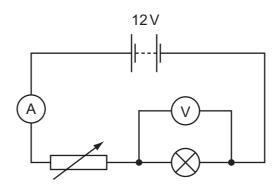
When the lamp brightness is low, the voltmeter reading is 2V and the ammeter reading is 2A.
