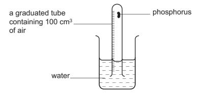
The initial volume of the air in the tube is 100 cm<sup>3</sup>.
