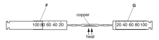
At the start of the experiment there is  $90 \text{ cm}^3$  of air in the apparatus. The air is passed backwards and forwards between gas syringes **F** and **G** over the heated copper. This is repeated until the volume stops decreasing. The gas is allowed to cool to room temperature and the final volume is measured.
