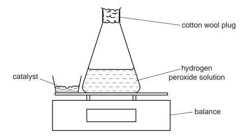
The manganese(IV) oxide is added to the hydrogen peroxide solution and the mass of the flask and contents recorded every 30 seconds. This is **experiment 1**.
