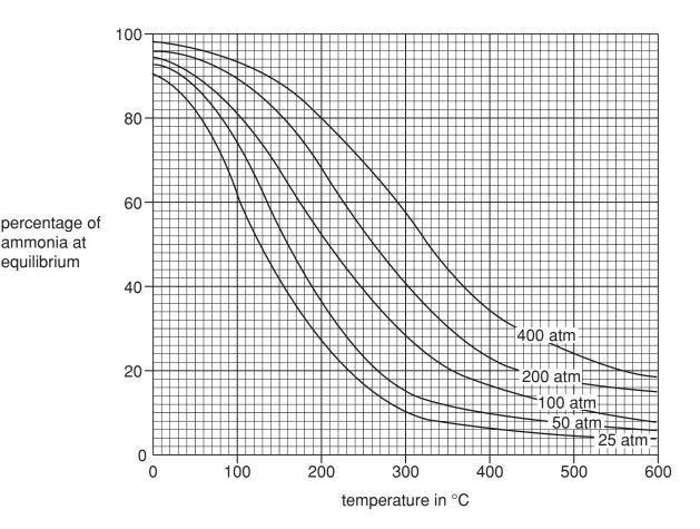
The reaction requires the use of a catalyst, which operates most efficiently within the temperature range 280 - 450 °C.
