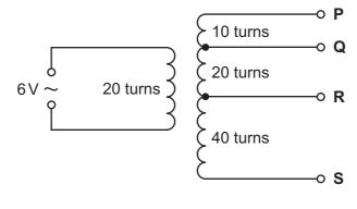
Between which terminals will the output be 12V?
