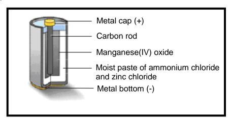
The paste of ammonium chloride reacts according to the following half-reaction:
