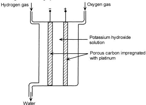
In the fuel cell, the hydrogen gas reacts according to the equation:
