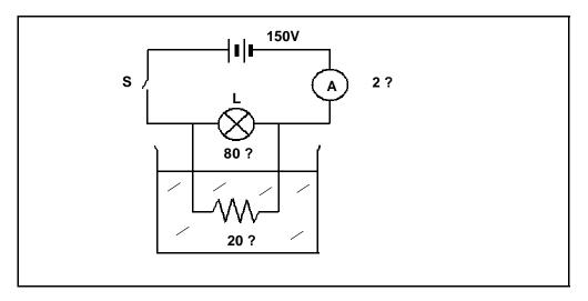
**L** is a bulb, which shows when the circuit is completed (closed). The water starts boiling 3 minutes after switch **S** is closed. The ammeter has a resistance of 2 ?.
