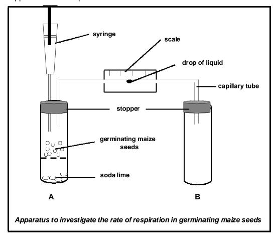
The rate of respiration was determined by measuring the distance travelled by a drop of liquid in a capillary tube. Movement of the drop of liquid is caused by a decrease in pressure in the container.
