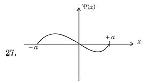
The figure shows one of the possible energy eigen functions  $\Psi(x)$  for a particle in infinite square well potential V = 0 for |x| < a and V =  $\infty$  for |x| > a. If the energy eigenvalue of this state is 2 eV, what is the energy eigen-value of the particle in the ground state ? (A) 0 eV
