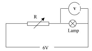
The above circuit can be used to vary the brightness of the lamp
