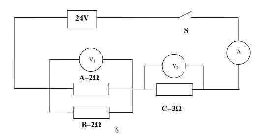
When switch S is closed, V<sub>1</sub> reads 6V. Calculate,
