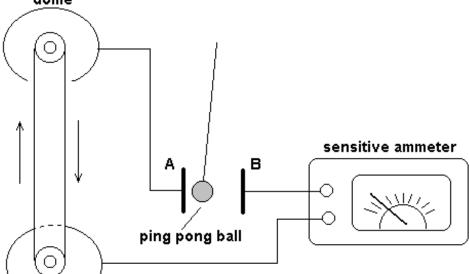
As the experiment is set going the charge that collects on the dome moves to plate A and the metal covered ping-pong ball swings between the 2 plates. The sensitive current meter shows a weak electric current flowing.
