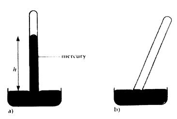
This instrument is used to measure atmospheric pressure.
