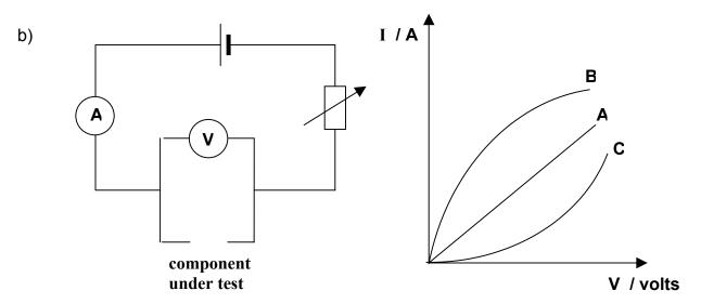
The circuit above is used to find how the current flowing through an electrical component varies with the voltage across its ends. The graphs known as characteristics show this for three particular electrical components.
