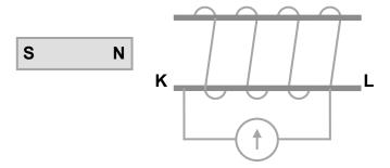
When the magnet is pushed into the coil, the **galvanometer pointer** deflects **clockwise.**
