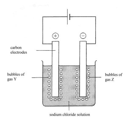
If a few drops of universal indicator are added to the solution before electrolysis starts, the indicator is green.
