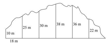
At equal intervals of 18 m along the dam, perpendicular measurements are made to the opposite bank, as shown on the sketch.
