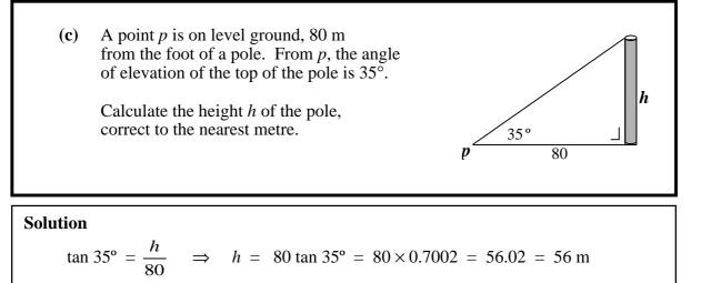
•  $\tan 35^\circ = \frac{h}{80} \dots 8$  marks.  $h = 80 \tan 35^\circ$  or  $0.4838 = \frac{h}{80} \dots 11$  marks.  $h = 56.02 \dots 14$  marks. h = 56 m  $\dots 15$  marks.
