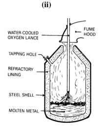
(i) Mild Steel is produced in the **Basic Oxygen Furnace**. The charge consists of scrap iron and steel together with lime and molten pig iron. Oxygen is blown at the surface of the molten charge from a water cooled lance which is lowered through the mouth of the furnace. Impurities in the charge are oxidized and form a slag on the surface. At the end of the blow, the steel is poured off through a tapping hole followed by emptying the slag through the mouth of the furnace.
