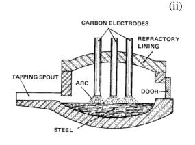
High Carbon Steel is produced in the **Electric Arc Furnace**. Cold scrap iron or steel make up the majority of the charge together with small amounts of lime and carbon. Heat for this furnace is by an electric arc created between carbon electrodes and the charge. The lime combines with impurities producing slag. When the correct composition of steel is achieved the slag is removed and the steel tapped from the furnace.
