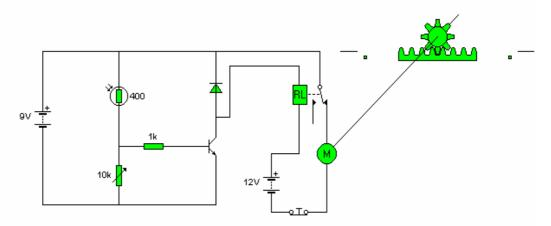
The motor driving the pinion is driven by the low voltage circuit. When light flow to the light dependent resistor is interrupted, by a person arriving at the doorway, the resistance is reduced. The transistor is activated switching on the relay. The motor circuit is then switched on causing the pinion to move the rack and open the door. The push-to-break switch will prevent the pinion running off the rack.
