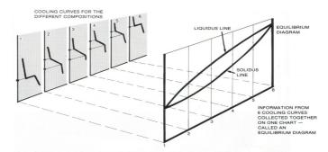
If the information from a range of cooling curves for different combinations of the alloy is collected on one chart, a thermal equilibrium diagram is formed.
