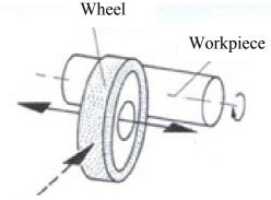
reciprocate and the wheel head can move towards the workpiece. Tapered work can also be carried out.
