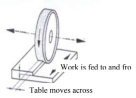
smooth surfaces are produced. The grinding wheel rotates and the workpiece, usually held in a magnetic chuck, is fed to and fro continuously. At the end of each stroke, the table is moved across the wheel by a small amount. The grinding wheel can be lowered to take a new cut.
