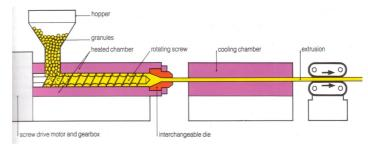
The extruded products can be cut into lengths or coiled. Polythene, PVC and nylon are commonly extruded.
