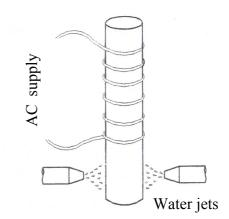
leaves the outer surface hard. The frequency of the current determines the depth of heating and the depth of hardening. Induction hardening is used on the slideways of a lathe.
