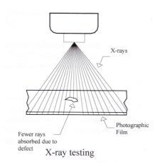
Radiation from an x-ray tube is passed through the weld. If no defects are present, the amount of absorption is uniform across the area exposed to the x-ray beam. If a defect is present in the weld, a smaller amount of rays is absorbed giving a variation in the intensity of the emergent beam. This can be detected by placing a photographic film on the side of the material opposite the radiation source. On a negative film, the defect shows as a dark spot.
