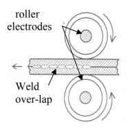
The time interval is controlled so that these spots overlap by approx. 40% of their length along the seam.
