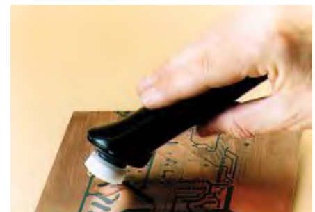
Flux being applied to a PCB
