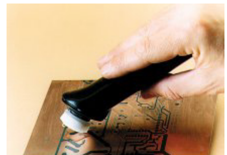
Flux being applied to a PCB
