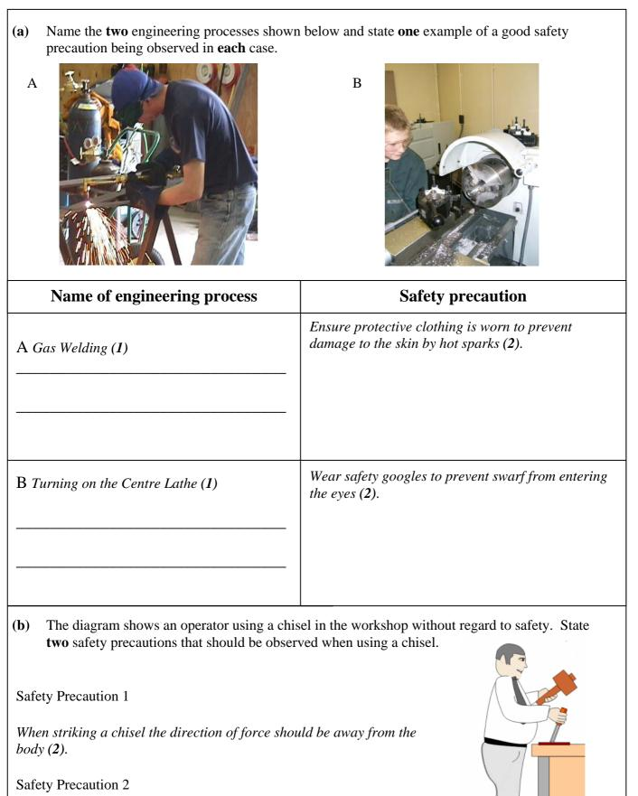
Safety gooles should be worn to prevent any waste metal from entering the eye (2).
