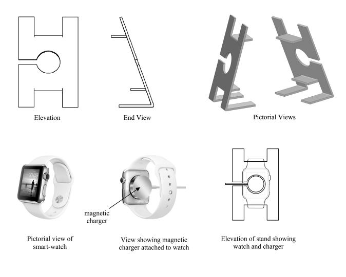
(i) Make a well-proportioned sketch of a **development** of the stand.Indicate clearly on your sketch the position of all cutting and bend lines.
