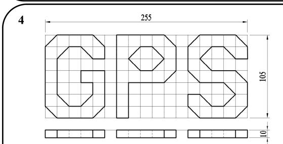
The figure shows the elevation and plan of the initials of a satellite navigation system. The grid in elevation is made up of 15 mm squares.
