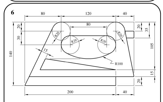
A design for an **electric iron** is shown. Reproduce the given figure, showing clearly all constructions and points of contact.
