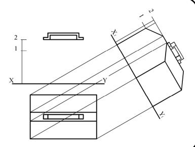
11 Using the grid provided, **sketch** the orthographic views indicated by the arrows.
