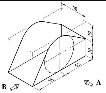
The figure shows the outline of a **bucket** for a mechanical digger. Draw:
