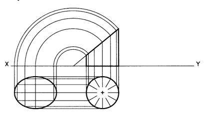
11. The elevation and plan of a ring are shown. Draw a <u>freehand</u> pictorial sketch of the ring in the space provided.
