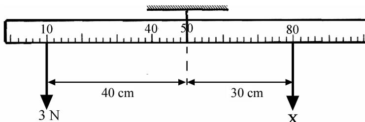
A uniform metre stick, suspended at its mid-point is balanced as shown.
