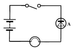
Explain why the lamp does not light when the switch is closed, assuming that all of the components are in working order. (6)
