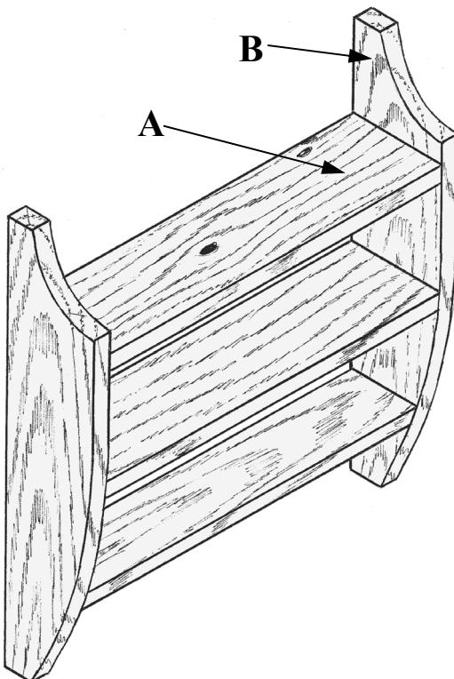
2. The diagram shows a pictorial drawing of a small display shelf. All material is **15mm** thick.
