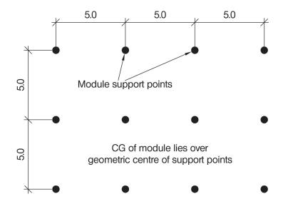
FIGURE Q8-2 : Plan showing position of required module support points
