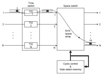
Student Bounty.com The transmission of signals carried out from sender to receiver through multiplexer in and de multiplexer output. The reverse communication also similar. Thus a hybrid arrangement is needed to isolate the transmitted signal from the received signal. The basic function of the time switch is to delay information in arriving time slots until the desired output time slot occurs.
