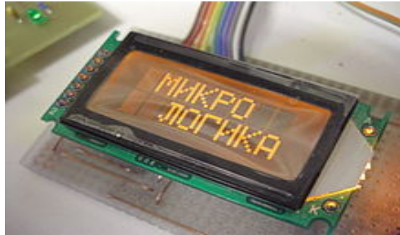
Amber backlight on a HD44780 display
