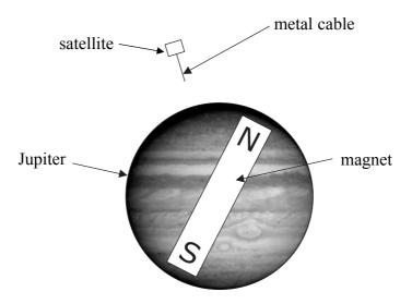
A satellite with a long metal cable hanging from it could generate electricity as it moves through the magnetic field of Jupiter.
