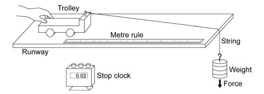
After releasing the trolley student **A**, measured the time it took for the trolley to travel 1 metre.
