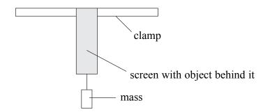
(a) Different masses are attached to the bottom of the object.
