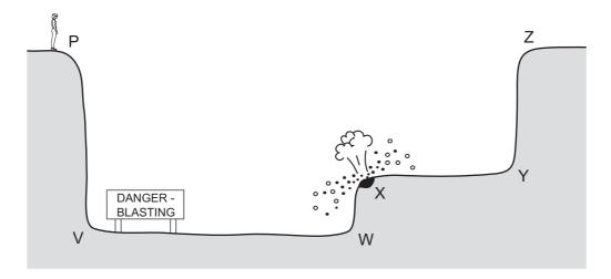
After the explosion, she hears two bangs. One bang is heard a fraction of a second after the other. The second bang is an echo.
