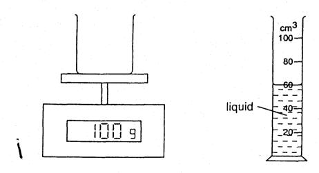
When all the liquid is poured into the beaker, the balance reading changes to 140 g.
