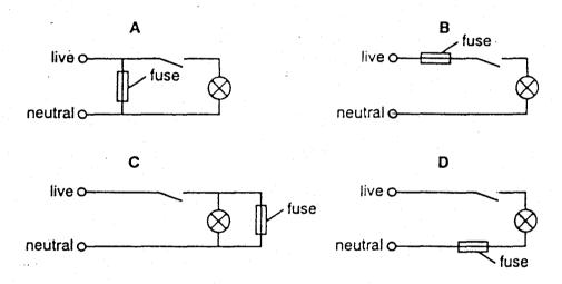
33 An electric kettle takes 12 A of current from the mains supply. When the kettle's cable needs to be replaced, a 5 A cable is used that was originally attached to a small lamp. The original plug and fuse from the kettle's cable are used.
