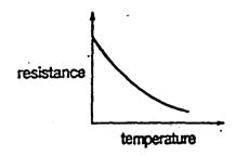
As the thermistor becomes cooler, what happens to its resistance and to the reading on the voltmeter?
