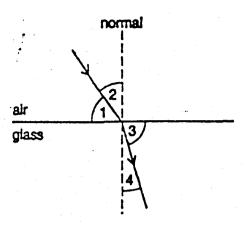
Which numbered angles are the angles of incidence and refraction?
