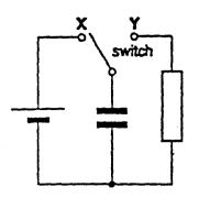
What will be happening to the capacitor when the switch is at X and when it is at Y?
