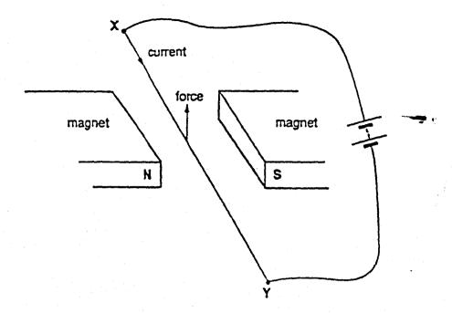
If the north and south poles exchange positions, in which direction will the force on the wire act?
