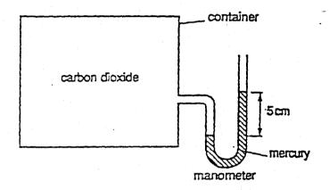
Which statement correctly describes the pressure exerted by the carbon dioxide?
