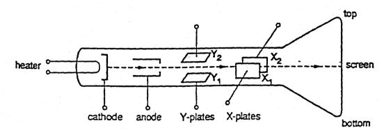
In the cathode-ray tube, what must be done to deflect the electron beam upwards?
