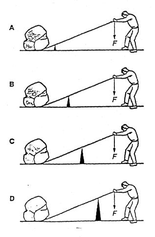
Which pivot position allows the force F to be as small as possible?
