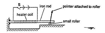
After the switch S is closed, what is the movement of the pointer and what is the magnetic state of the rod?
