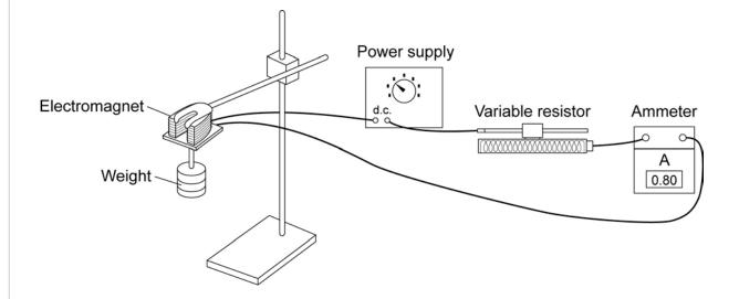
For different values of I and n the student measured the maximum weight supported by the electromagnet.
