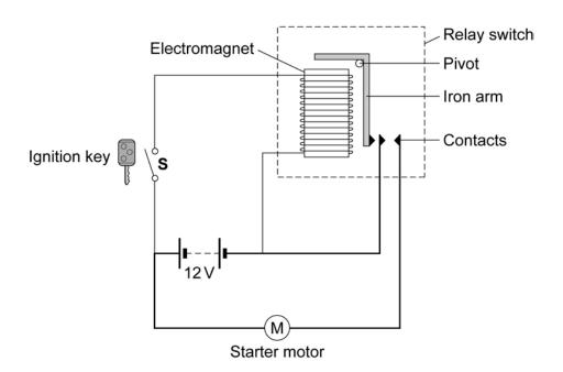
2 (e) (i) Explain how turning the ignition key causes the starter motor to work.
