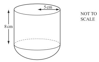
The shape of the toy is a cylinder of radius 5 cm and height 8 cm on top of a hemisphere of radius 5 cm.
