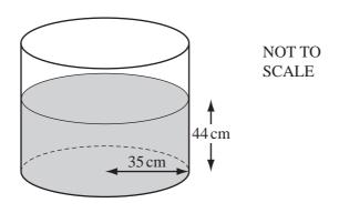
A cylindrical tank, with radius 35 cm, is filled with water to a depth of 44 cm.
