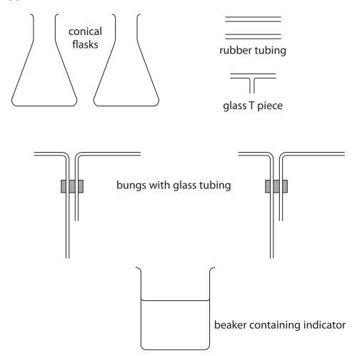
The apparatus is not drawn to scale.
